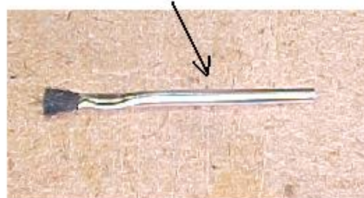
Acid brush used for melting clearance holes in Coroplast
