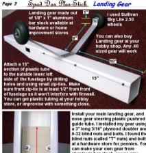
guide tube. I installed my gear using a 3" long 3/16" plywood doubler and 6-32 blind nuts and bolts. I found the blind nuts (called "T" nuts) and bolts at a hardware store for pennies. You aluminum bar stock, or use any hobby store bought .40 sized gear. If you are building your plane as a hand launched 3 channel combat plane, simply disregard this whole page.
