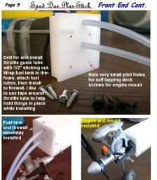
Take care not to intersect fuel lines or engine mout screws with firewall screws! Make sure there is foam between firewall and tank in case screws protrude through rear of firewall. Exact positioning of engine on firewall is not critical, make sure steering arm is not obstructed!
